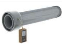
8 Nondestructive testing of welded joint (flaw detection)
