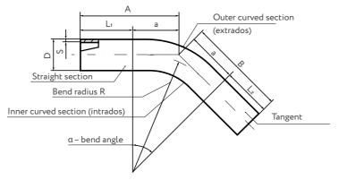
OD - outside diameter; S - wall thickness; R - bend radius; a - construction length of the bent section; L, L1 - tangent length; A, B - construction lengths. The bends are manufactured with bend angles from 1° to 90° with 1° increments. By agreement with the customer, bends with straight sections of any length can be manufactured.
