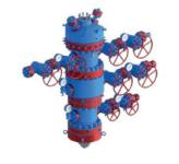
Designed to hook up service and casing strings as well as tubing in a single split body without reassembling the blowout preventer. Unitized wellhead equipment with protective ErNiCrMo-3 (Inconel 625), 06Kh15N60M15, or OKAutrod 309L (Kh25N13) coating against CO2 corrosion on the internal surface contacting the operating medium.
