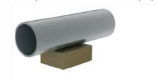
16. Magnetic particle and ultrasonic inspection of both pipe ends
