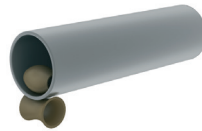
4. Post-bending of the longitudinal plate edges
