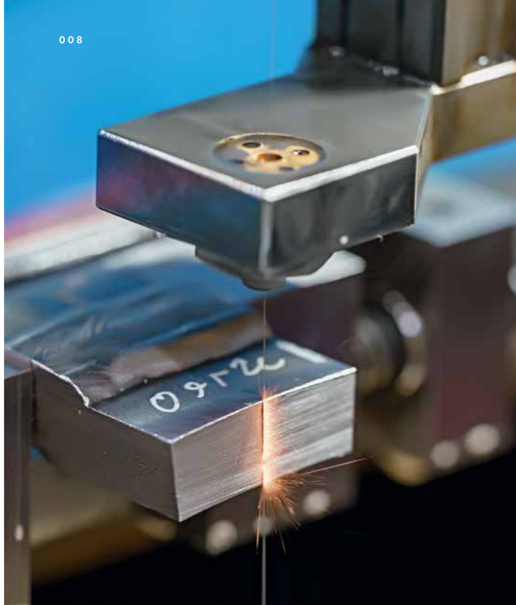
Electrical discharge machining prepares a specimen for mechanical tests
